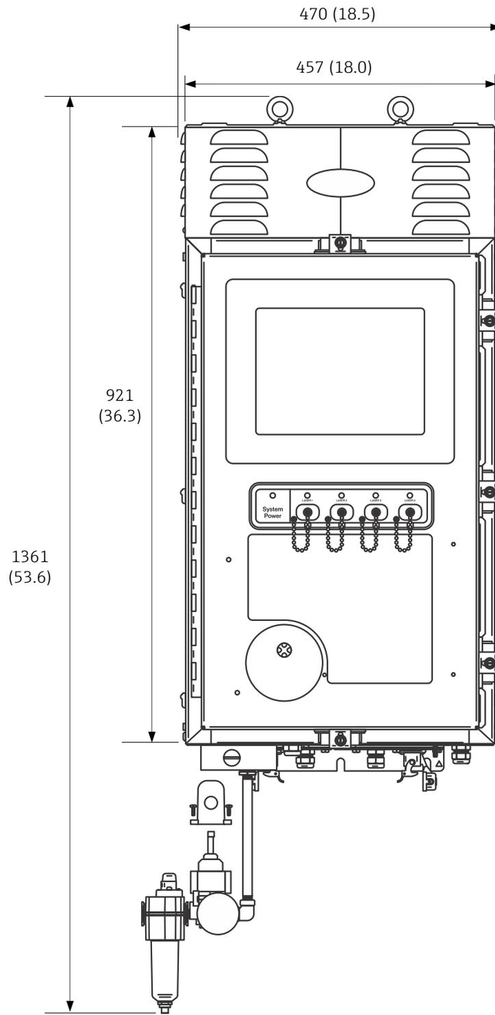
Figure 9. Raman Rxn5 front view. Dimensions: mm (in)
