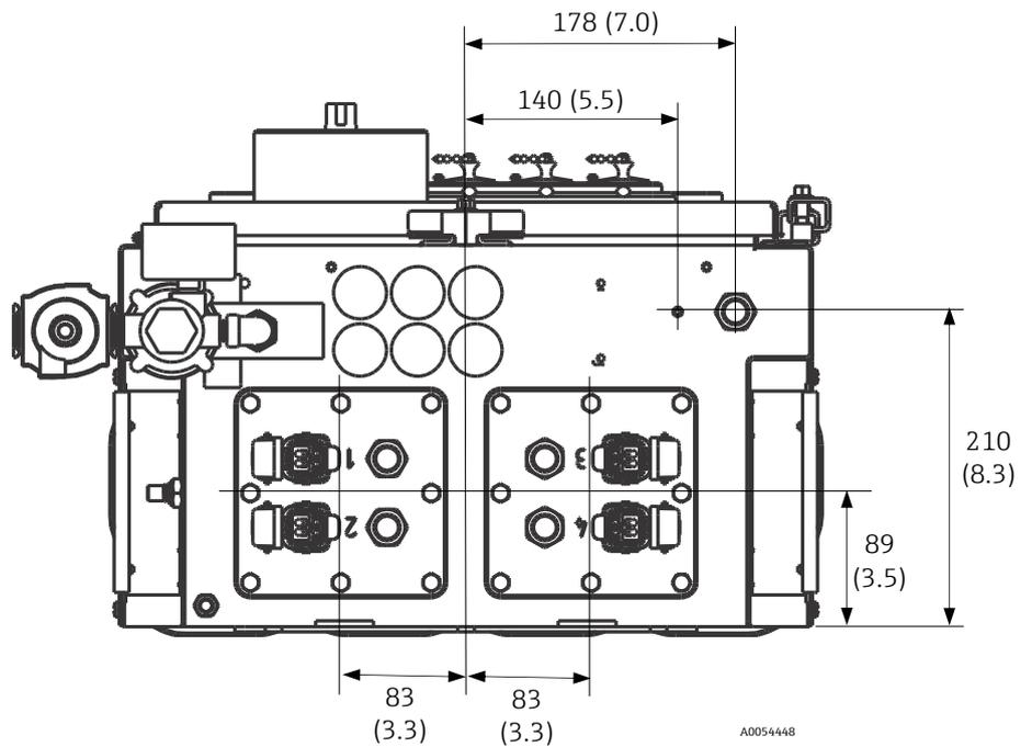
Figure 12. Raman Rxn5 bottom view. Dimensions: mm (in)
