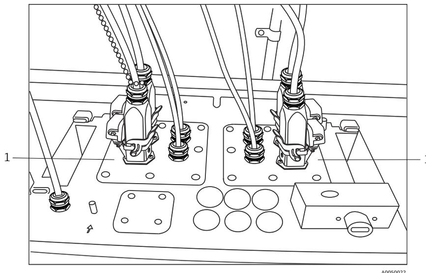
Figure 7. I/O panels provide sampling probe connections (1)
