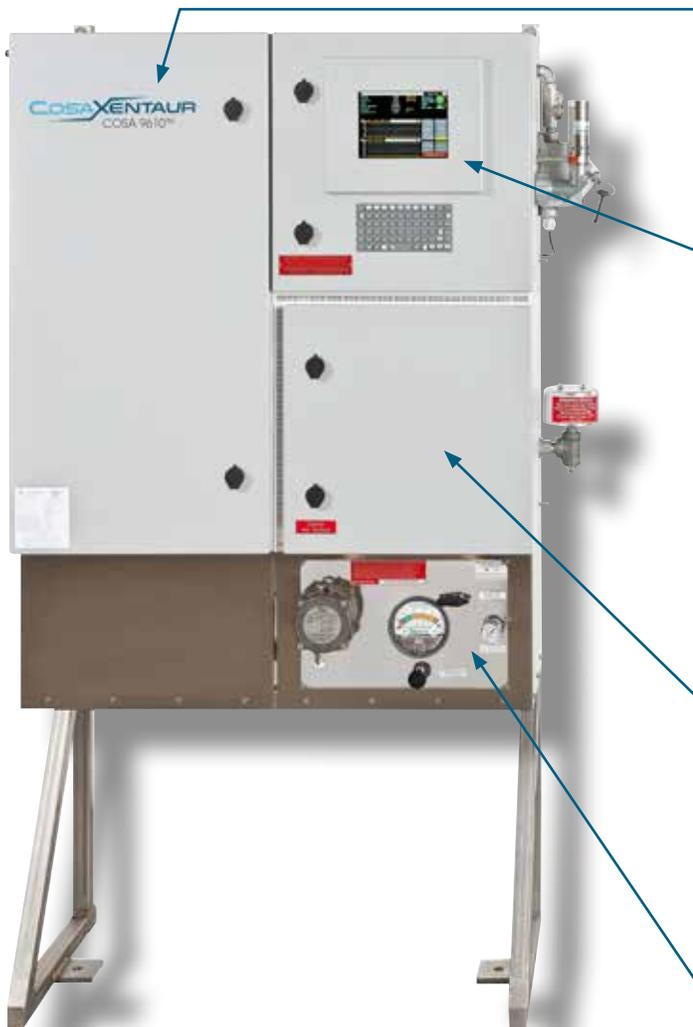
The **gas mixing compartment** contains sample conditioning and the gas mixing system. Components in this compartment are intrinsically safe. The gas mixing compartment is heated to avoid condensation of heavier gas constituents.
